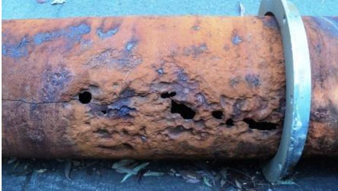
Figure: Corroded pipe section (Courtesy of Hunter Water)
