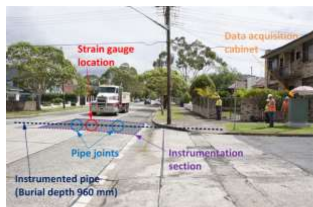
Figure 1: Layout of the pipe testbed
