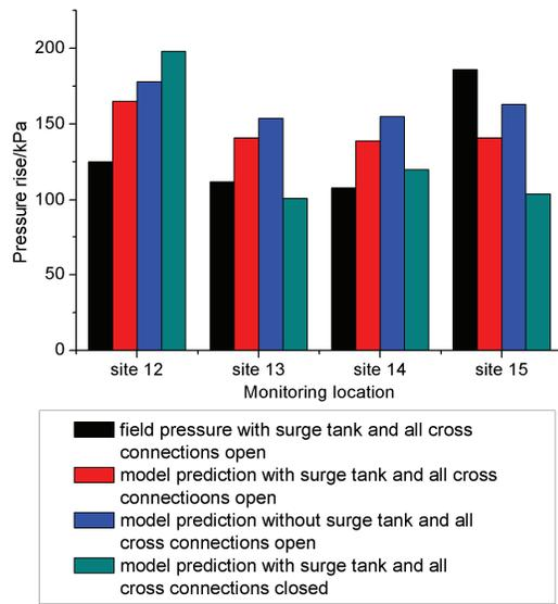
Figure 7. Comparison of pressure rise during different scenarios and monitoring location
