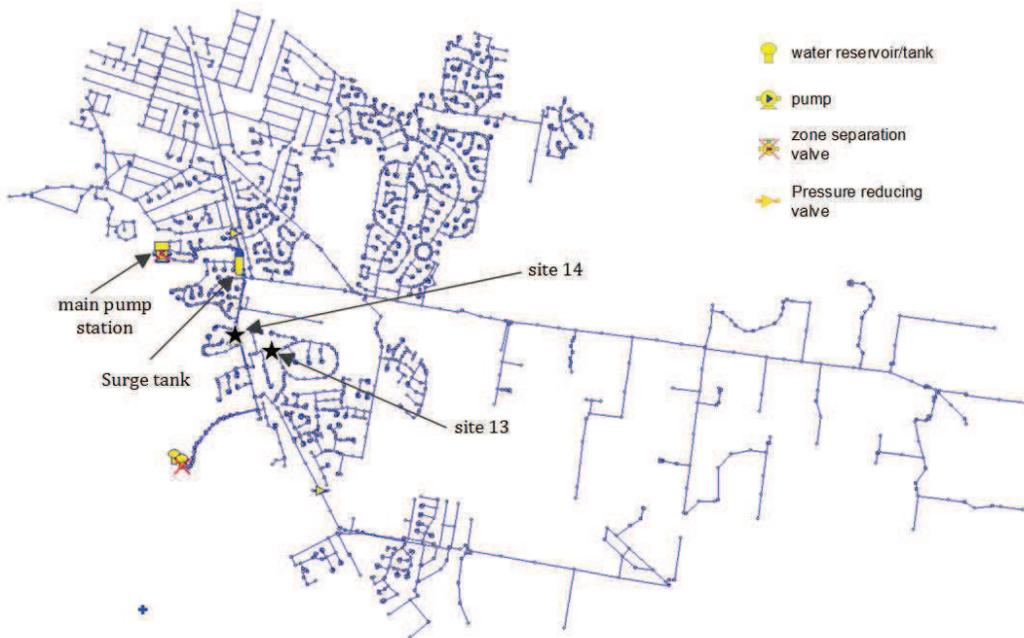
Figure 3. Pressure transient numerical model developed for Rosedale Grove section
