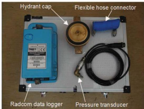
Figure 1. Radcom pressure transient monitoring data logger
