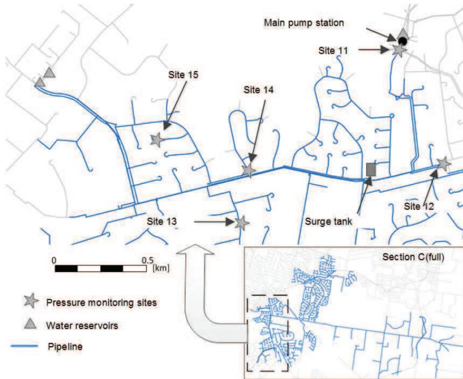
Figure 2. Pipe network and pressure monitoring sites
