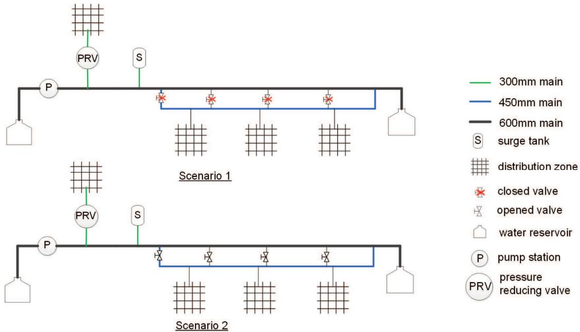
Figure 4. Two different scenarios monitored in Rosedale Grove pressure monitoring program
