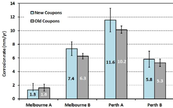
Figure 10. New and old coupon rates of corrosion.
