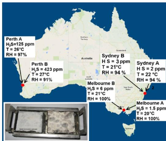
Figure 1: Location of field sites used in the study and conditions present at those site. Inset: coupon pair in sample holder.
