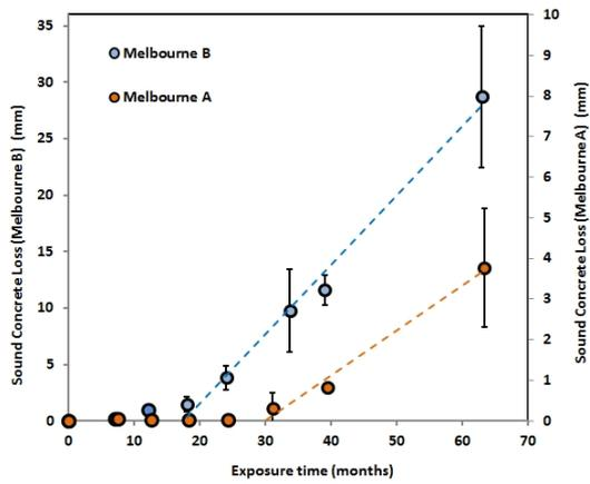
Figure 5. Melbourne new coupon losses.
