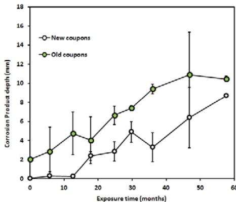
Figure 11. Depth of corrosion product layer on Perth B new and old coupons.
