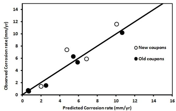
Figure 13. A comparison of predicted and observed corrosion rates. The diagonal lines represents perfect agreement.
