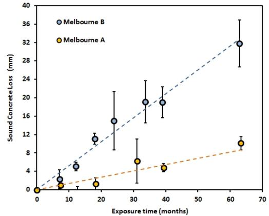
Figure 7. Melbourne old coupon losses.
