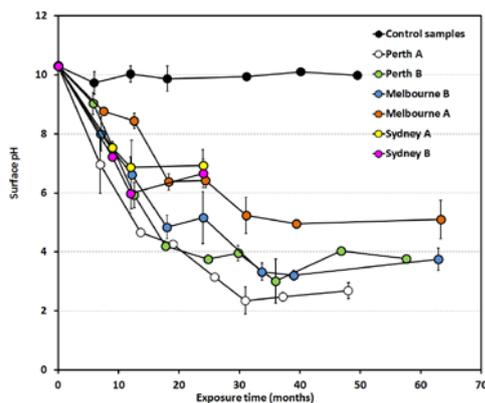
Figure 3. Evolution of surface pH of new coupons.
