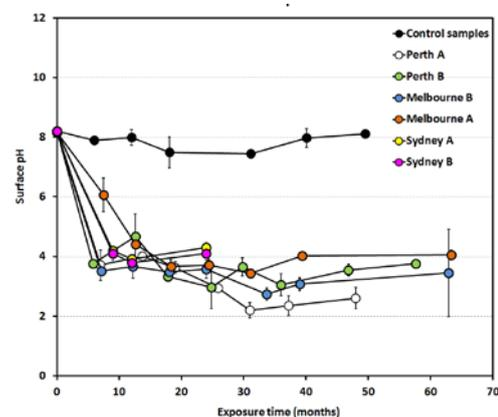
Figure 4. Evolution of surface pH of old coupons.
