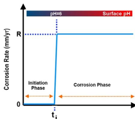
Figure 12. Bi-linear representation of the concrete sewer pipe corrosion process.
