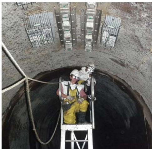
Figure 2: Samples being mounted along the crown of the Melbourne A sewer.
