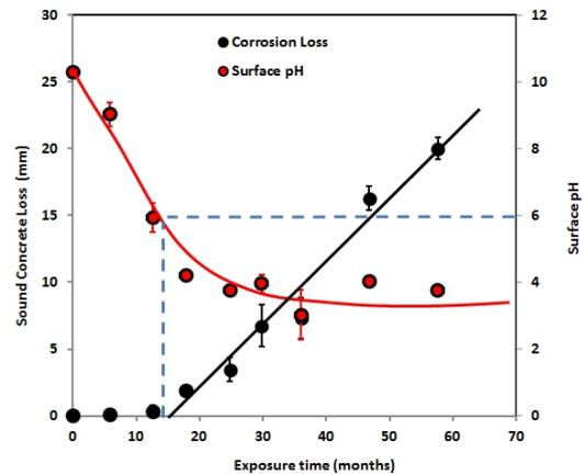
Figure 9. The onset of corrosion losses at pH=6 (Perth B).
