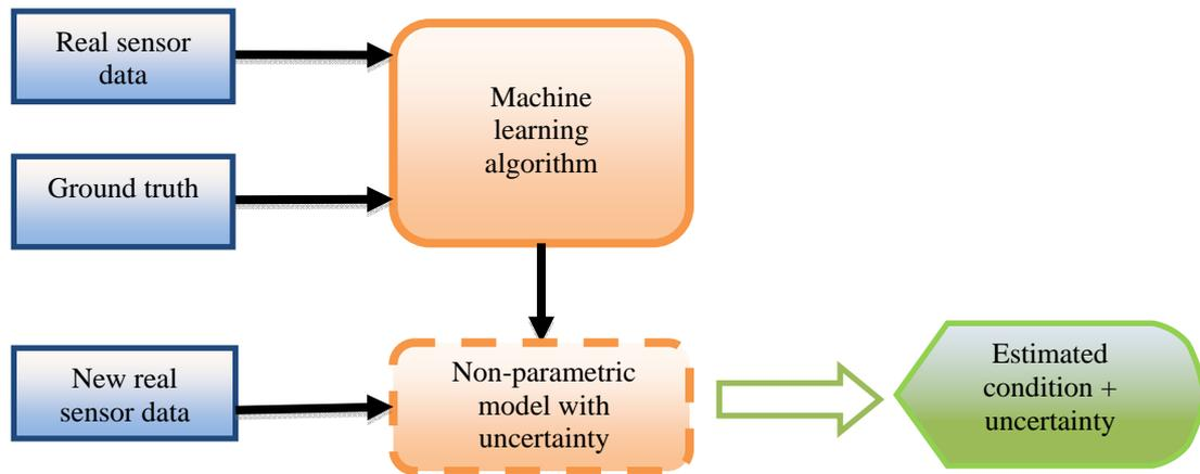
**Figure 9.** Diagram of the machine learning approach using Gaussian process regression.
