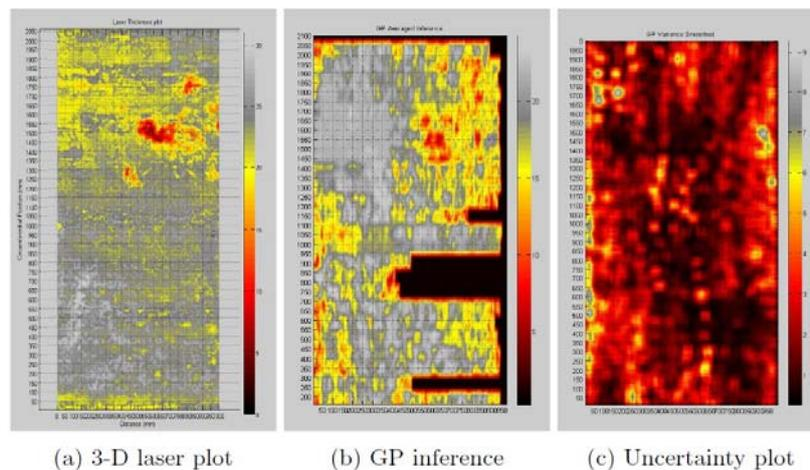
**Figure 10.** Comparison of real and predicted depth profile for MFL data.
