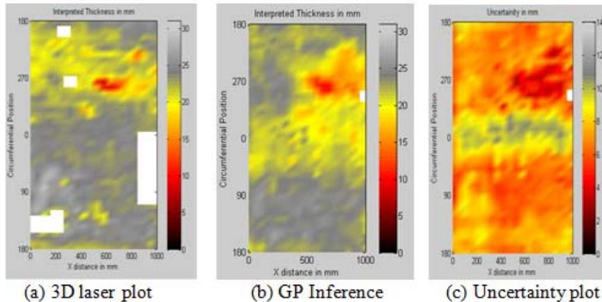
**Figure 11.** Comparison of real and predicted depth profile for BEM data.
