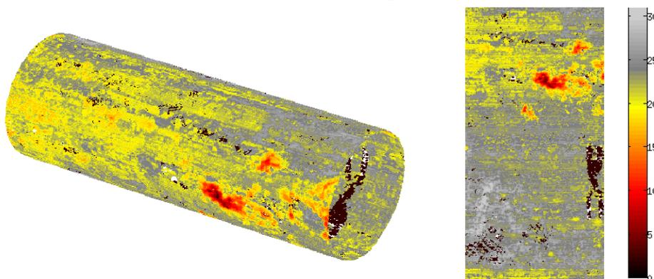
b) Thickness plots obtained through the UTS algorithm
