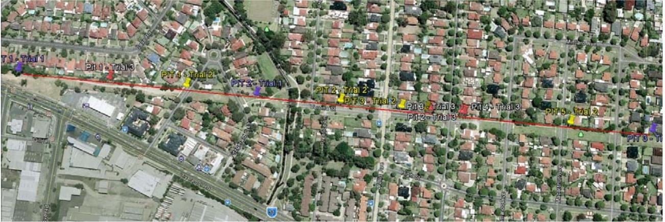
**Figure 1.** Google Earth (top-view) image of 1 km of Sydney Water’s test-bed. Excavation pits for research run 1 are shown in purple, for research run 2 are shown in yellow and for research run 3 are shown in red.
