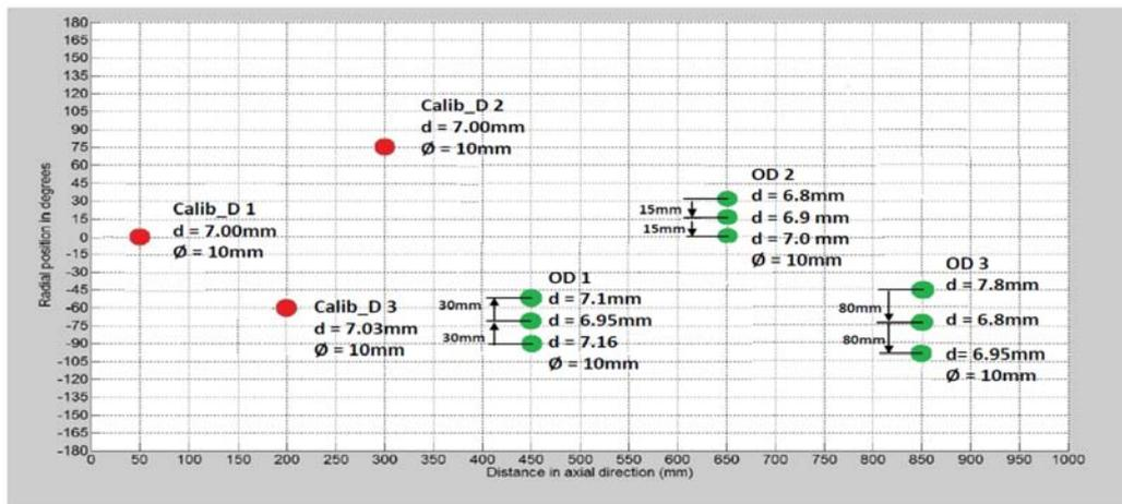
b) Example of calibration defects
