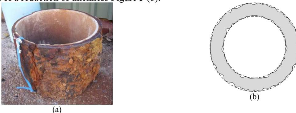
**Figure 3.** General corrosion: (a) field observation and (b) idealisation of general corrosion
