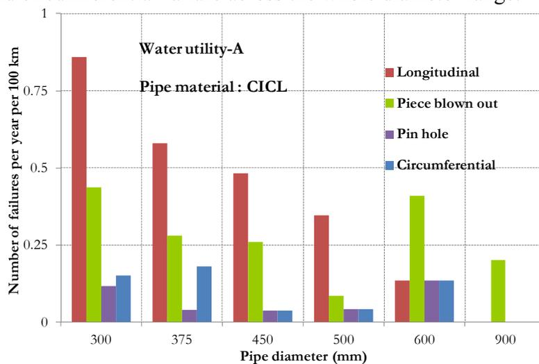
(a) Cast iron cement lined pipes (CICAL)
