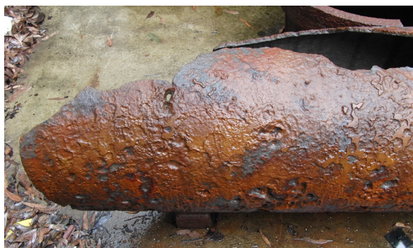
Figure 1 Exterior corrosion of a 110 year old cast iron water main with graphitised zone removed
