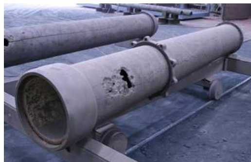
Figure 8 Photograph of corrosion by different soils in contact with pipe. Note that the corroded area is located on the bottom of the pipe when the pipe was in service.
